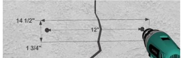
**Step B:** Using 1/2" masonry bit drill both holes into concrete approximately 4" deep.
