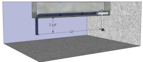
\*Note: A minimum 5" slab is recommended for Mechanical Stitch installation. For shallower slab thicknesses, drill the anchor hole and install and tighten the nut. Once tightened the threaded shaft may extend upward and can be ground down flush with the top of the nut. Chip out niche bottom flat for optimal installation performance.
